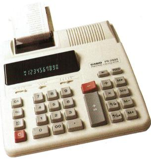
■ Full decimal system - floating, fixed (0-4) with round-off or cut-off and ADD mode ■ Sub total/total/grand total ■ Mark-up/mark-down ■ Item count ■ 3 digit comma markers ■ Double zero key ■ 1.6 lines per second ■ Mains powered.
